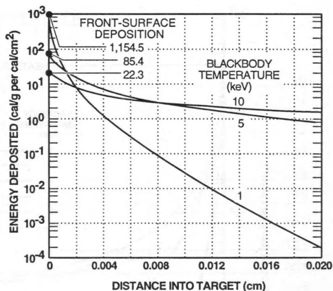
Figure 7.9. ANISN Deposition Profile for Iron at Blackbody Temperatures of 1, 5, and 10 keV (Incident Fluence = 1 cal/cm<sup>2</sup>).
